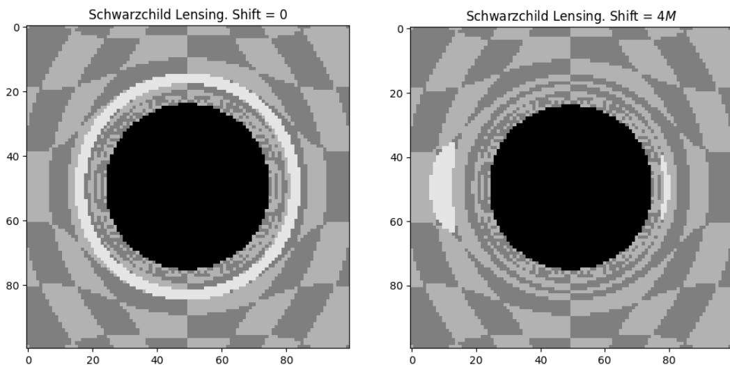
Figure 5: Gravitational lensing for the Schwarzschild metric. The bright patch behind the black hole is shifted along the Y axis.
