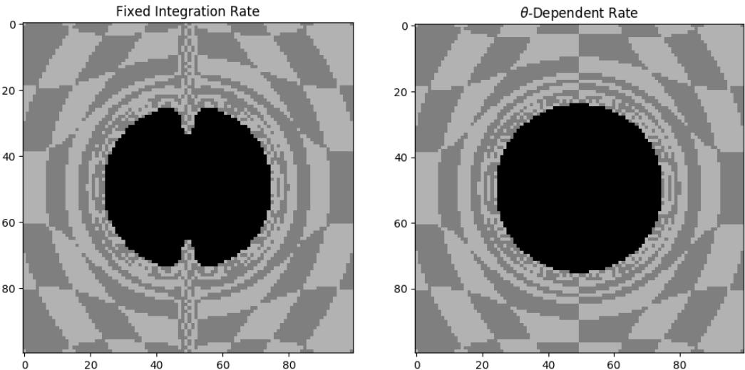
Figure 3: Images with the Schwarzschild metric (without the bright patch). Left: the step size is constant at 0.05. As rays pass close to the  $z$  axis, the small values of  $\theta$  cause errors in numerical integration. Right: errors are removed if step size is reduced.
