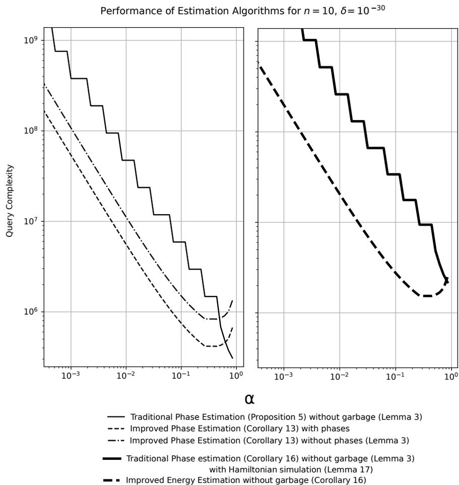
Figure 5.5: Performance of estimation algorithms presented in this chapter. Phase estimation algorithms are presented with slim lines on the left, and energy estimation algorithms are presented with thick lines on the right. The zig-zag behavior of phase estimation is explained by the method by which Proposition 5.5 reduces  $\alpha$ : by estimating more bits than needed and then rounding them. Thus, the  $\alpha$  achieved by phase estimation is always a power of two.
