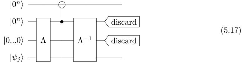
First, we consider the ideal case when  $\Lambda$  implements the map (5.16) exactly. If we use  $|\psi_j\rangle$  as input and we stop the circuit before the discards, we produce a state  $|\text{ideal}_j\rangle$ :
